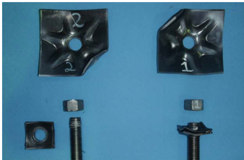
Figure 2. Y20 x 1.5 m Long Roof bolt assemblies after the test.
